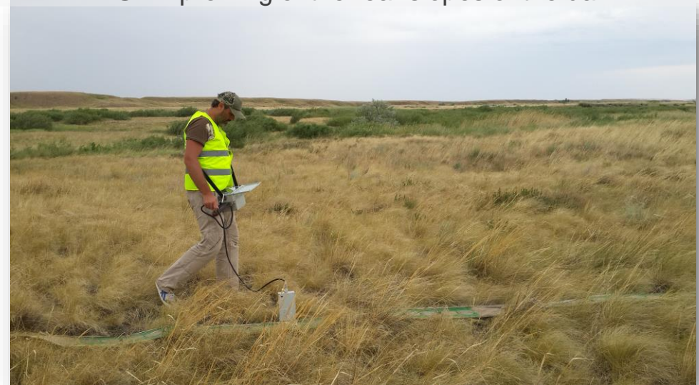
DGPR profiling of the rear slopes of the dam
